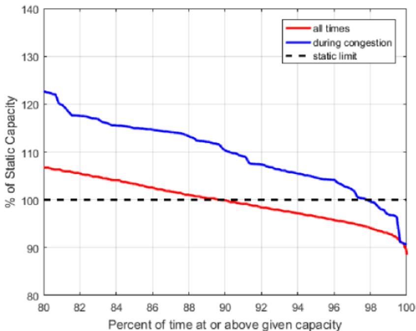
Figure 1: Modeled Capacity on Kansas Transmission Line<sup>11</sup>
